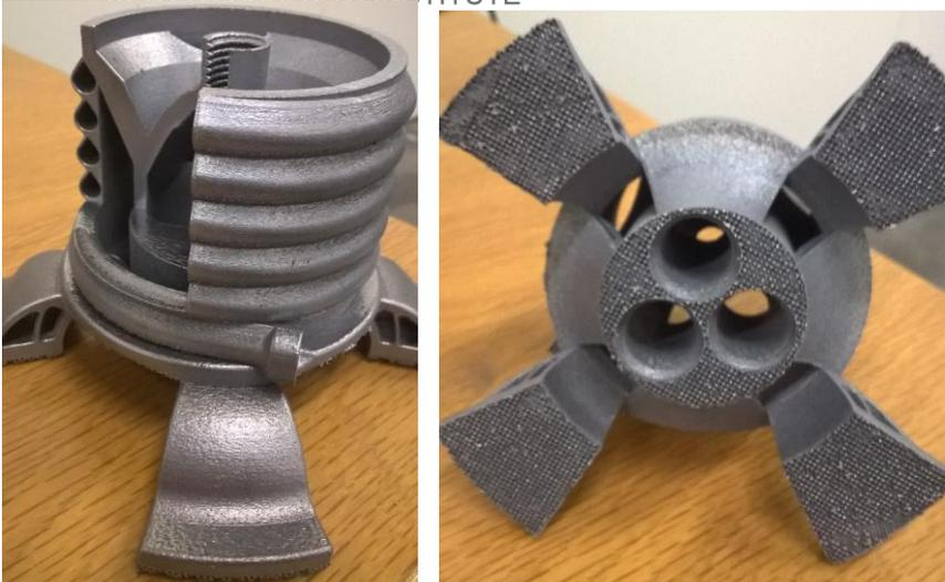
**Fig.11** Printed part: (a) AM part and (b) support structure of the AM part
