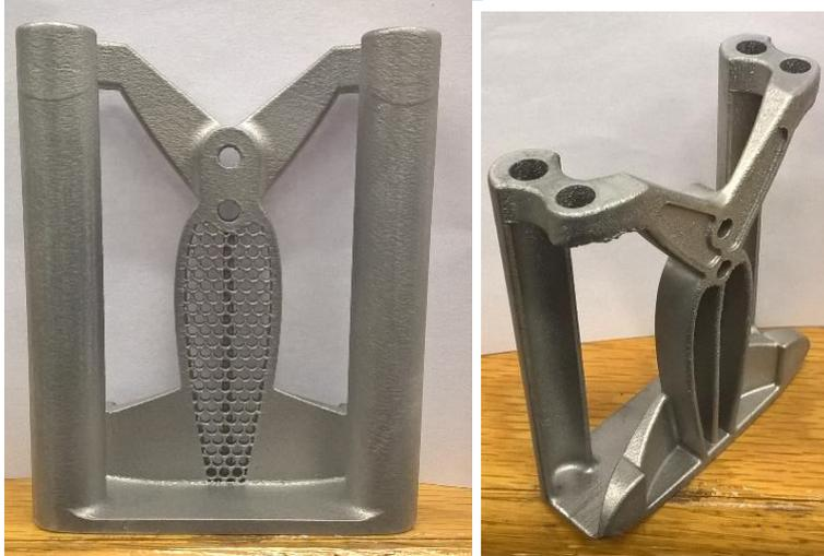
**Fig.8** Printed clamp after post-processing; (a) frontside view and (b) backside view.
